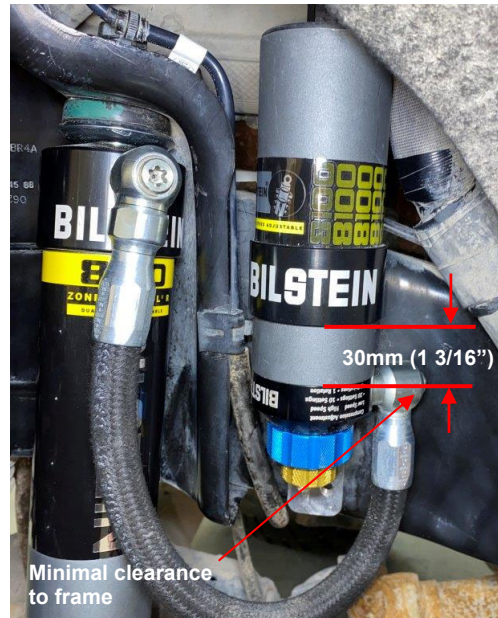
Left (Driver) DSA Reservoir Placement
