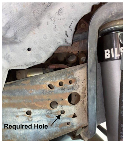
Right (Passenger) Side w/ Holes
