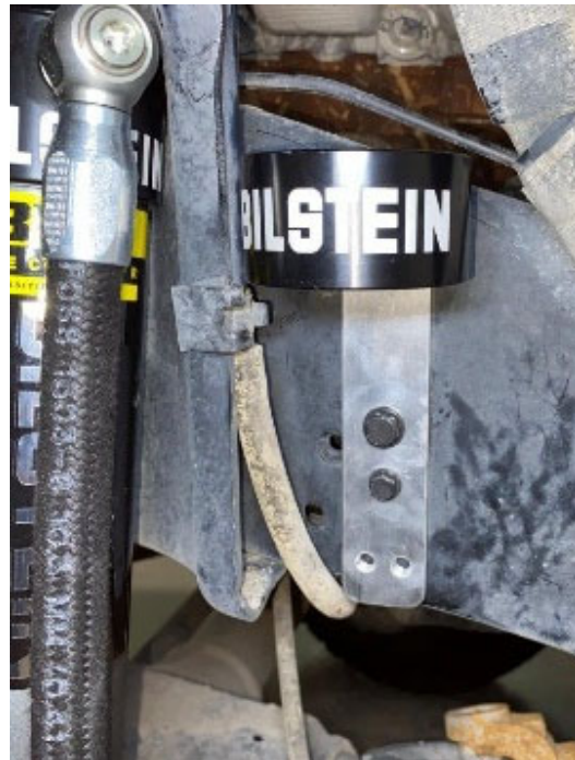
Left (Driver) Side Depicted – Holed Frame Vehicle and Installed Mount Plate
