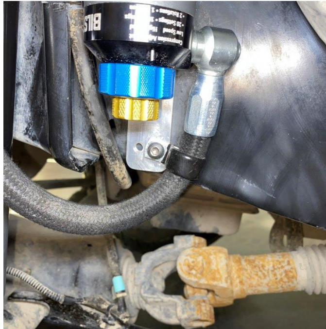
Left (Driver) Hose Clamp Install (DSA Pictured)
