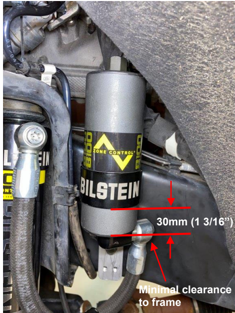
Left (Driver) Reservoir Placement
