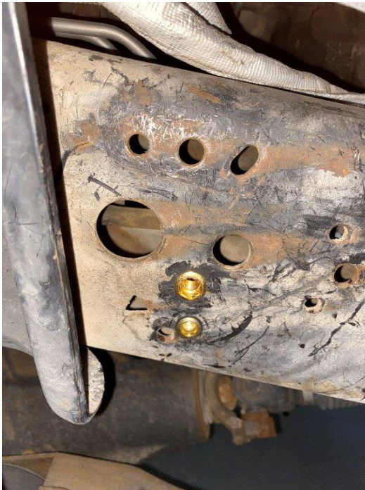
Left (Driver) Side Depicted – Holed Frame Vehicle and Installed Mount Plate
